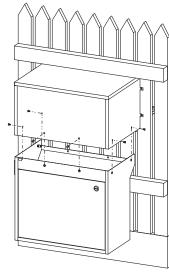
10. Open the rear door. Reach up inside the body, towards the front to secure the last 2 bolts.
