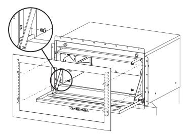
Detach the lower box from the upper box by unscrewing the 6 external bolts using the allen key supplied.
