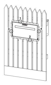
8. To re-attach the front panel, place the front panel into the body. Open the parcel door and secure with the 4 bolts previously unscrewed in step 1.
