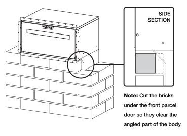
4. Complete the remaining brickwork around the letterbox. Finish any brick cleaning or rendering.
