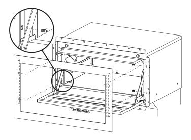
2. Build the brickwork up to the desired level and set the back box in place.
