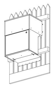
12. Re-attach the mounting bracket onto the underside of the letterbox loosely tightening the same 2 sets of nuts and bolts.
