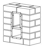
3. Once the brickwork and any rendering has been completed, attach the front panel by inserting the 4 x mounting studs through the corresponding holes in the back box.
