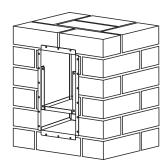
3. Once the brickwork and any rendering has been completed, attach the front panel by inserting the 4 x mounting studs through the corresponding holes in the back box.
