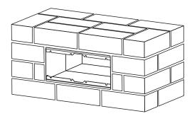
3. Once the brickwork and any rendering has been completed, attach the front panel by inserting the 6 x mounting studs through the corresponding holes in the front sleeve.
