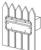
4. Attach the front panel by inserting its six mounting studs through the corresponding holes in the back box. Secure with the nuts provided.
