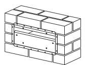
4. Once the brickwork and any rendering has been completed, attach the front panel by inserting its six mounting studs through the corresponding holes in the back box. Secure with the nuts provided.
