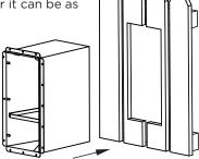
2. Slide the letterbox body in through the <u>front</u> of the fence. Screw it to the fence with the screws provided (for hardwood, its easier if you pre-drill the screw holes).
