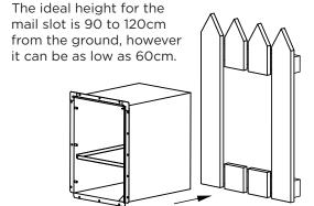
3. Slide the letterbox body in through the <u>front</u> of the fence. Screw it to the fence with the screws provided (for hardwood, its easier if you pre-drill the screw holes).
