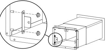
6. Attach mounting clips to the top and right side of the sleeve.
