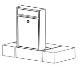
2. Complete the remaining brickwork around the letterbox.
