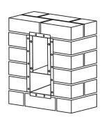
3. Once the brickwork and any rendering has been completed, attach the front panel and secure it from inside of the letterbox with the nuts provided.
