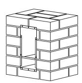
3. Once the brickwork and any rendering has been completed, attach the front panel and secure it from inside of the letterbox with nuts provided.
