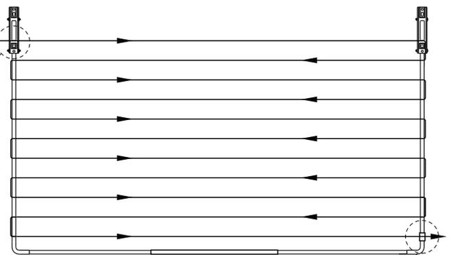
4. Thread the cord through the Line Tensioner as shown. Lift the clamping lever up before threading the cord. Push the lever down to clamp the cord.
