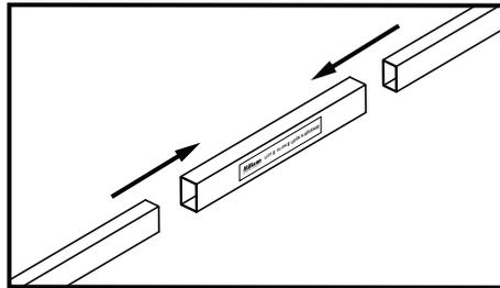
5. Spread the side arms slightly apart and insert the assembled front bar into the corners as shown right.
