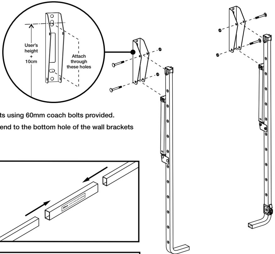
3. Fit the side arms to the top hole of the wall brackets using 60mm coach bolts provided.
