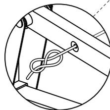
3. Progressively tighten each line, starting from the rear, working towards the front. Don't over-tighten or you will distort the side arms.
