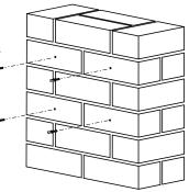
2. Mount the letterbox onto the brickwork with the spacers and screws provided.
