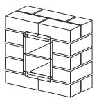
4. Once the brickwork and any rendering has been completed, attach the front panel by inserting its four mounting studs through the corresponding holes in the back box. Secure with the nuts provided.
