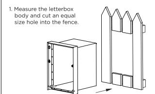
2. Slide the letterbox body in through the <u>front</u> of the fence. Screw it to the fence with the screws provided (for hardwood, its easier if you pre-drill the screw holes).
