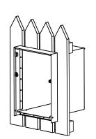
3. Attach the front panel using the bolts and nuts provided with the front panel (refer to the instruction sheet included with the Front Panel).
