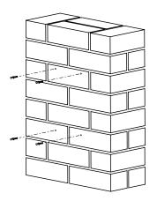
2. Mount the parcel letterbox onto the brickwork with the screws provided.
