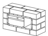
4. Once the brickwork and any rendering has been completed, attach the front panel by inserting its four mounting studs through the corresponding holes in the back box. Secure with the nuts provided.
