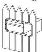
4. Attach the front panel by inserting its four mounting studs through the corresponding holes in the back box. Secure with the nuts provided.
