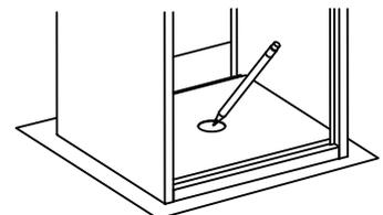
5. Drill a hole (10mm diameter x 70mm deep) into the concrete slab for the mounting bolt.
