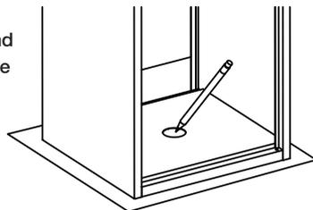
2. Drill a hole (10mm diameter x 70mm deep) into the concrete floor for the mounting bolt.
