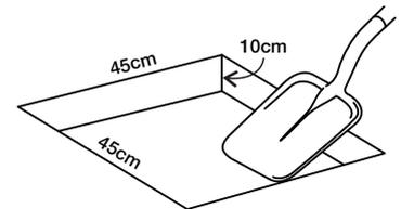
2. Fill hole with concrete.
