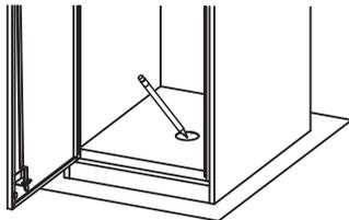
2. Drill a hole (10mm diameter x 70mm deep) into the concrete floor for the mounting bolt.
