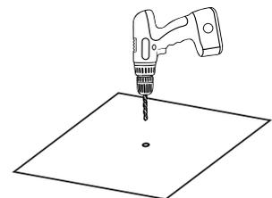
6. Place the letterbox back over the concrete hole just drilled. To bolt the letterbox to the concrete floor, refer to the steps below.
