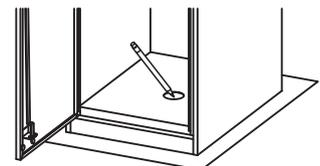
5. Drill a hole (10mm diameter x 70mm deep) into the concrete slab for the mounting bolt.
