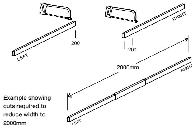
9. Assemble the front bar as shown in Detail B. Push the left and right bars fully into the centre bar until they hit the small indent in the middle of the centre bar.
