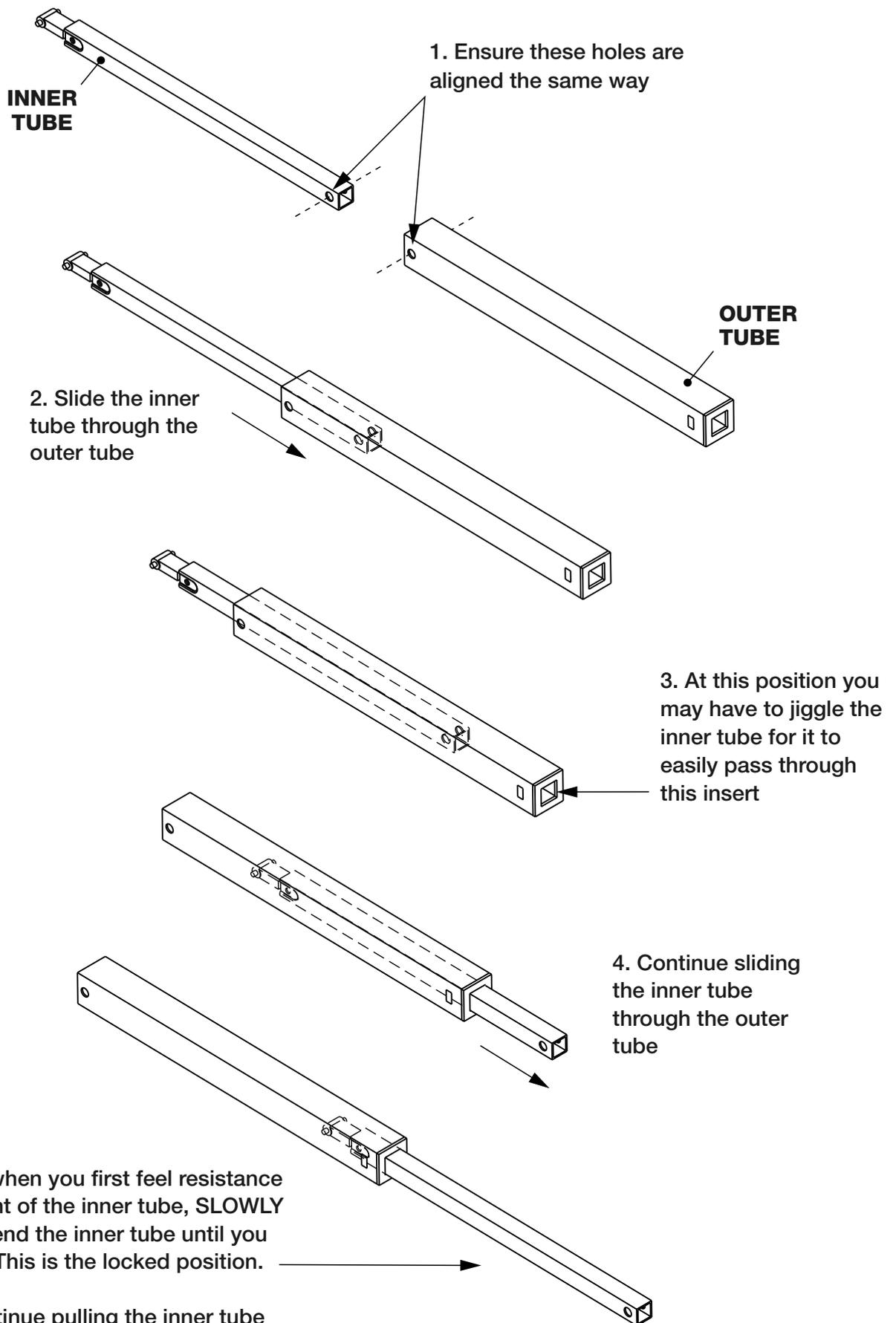
To unlock - continue pulling the inner tube outwards until you hear another click - this is the unlocked position.
