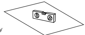
4. Place your letterbox onto the concrete slab and mark the mounting hole with a pencil
