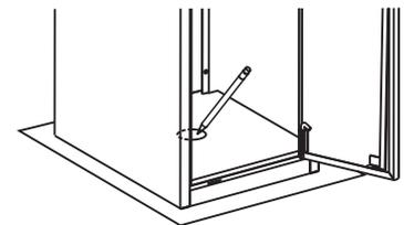
5. Drill a hole (10mm diameter x 60mm deep) into the concrete slab for the mounting bolt
