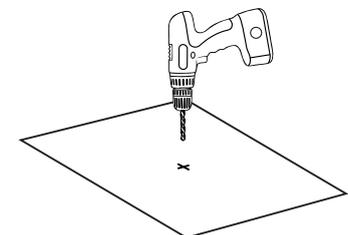
6. Bolt the letterbox to the concrete slab with the mounting bolt provided.
