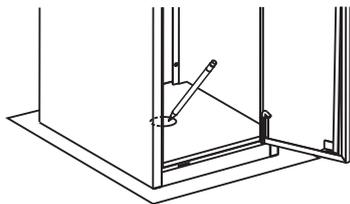
2. Drill a hole (10mm diameter x 60mm deep) into the concrete floor for the mounting bolt
